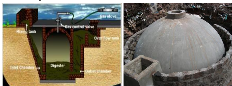
Gambar 2. Reaktor biogas tipe kubah tetap ( fixed dome type )
