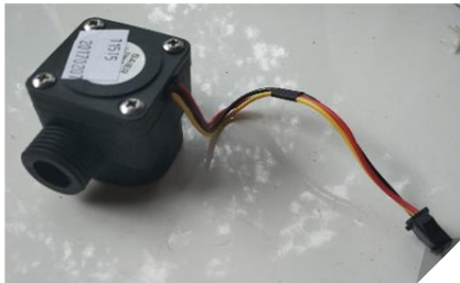
Gambar 6. YS-S201 Hall Effect Water Flow Meter
